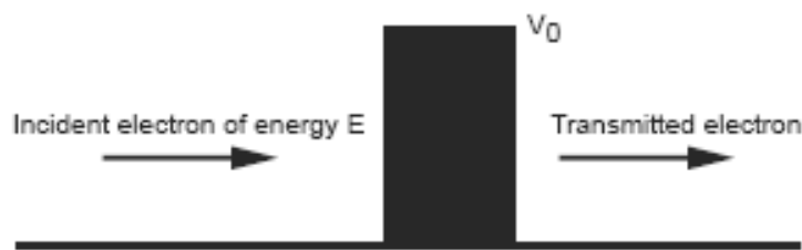
Figure 1.1 The basics of Tunnelling. An electron of energy E is incident on a barrier of potential V_0 . Classically, the electron is reflected when E < V_0 , quantum mechanically, there is a probability that the electron is transmitted through the barrier.
